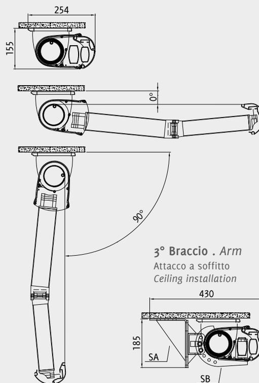
Inclinazione tenda a 3 bracci da 0° a 60° . Awning with 3 arms: inclination from 0° to 60°.
